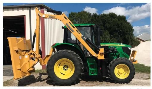
The District's new John Deere 6110M Boom Arm Mower is designed to mow canal banks and roadside ditches - it replaces the John Deere 6420 Boom Mower previously used by the District
